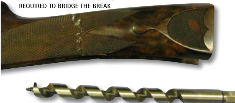
NOTE THE LENGTH OF THE BORING BIT REQUIRED TO BRIDGE THE BREAK
