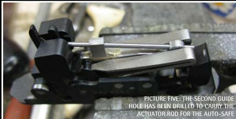
PICTURE FIVE: THE SECOND GUIDE HOLE HAS BEEN DRILLED TO CARRY THE ACTUATOR ROD FOR THE AUTO-SAFE
