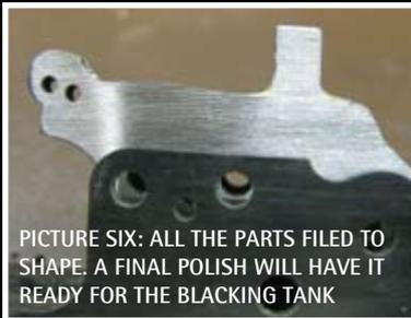
PICTURE SIX: ALL THE PARTS FILED TO SHAPE. A FINAL POLISH WILL HAVE IT READY FOR THE BLACKING TANK
