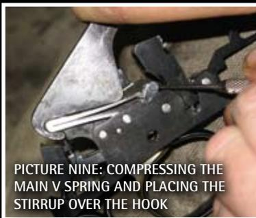
PICTURE NINE: COMPRESSING THE MAIN V SPRING AND PLACING THE STIRRUP OVER THE HOOK
