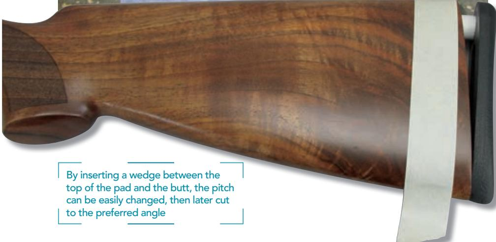
By inserting a wedge between the top of the pad and the butt, the pitch can be easily changed, then later cut to the preferred angle
